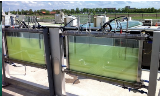
Flat panel reactor for outdoor microalgae cultivations at AlgaePARC (The Netherlands)
